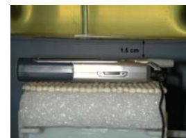
Figure 14.13 Body SAR Test Setup -- w/o Holster --
