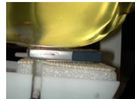
Figure 14.8 Right Head SAR Test Setup -- Cheek / Touch Position --
