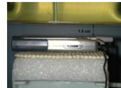
Figure 14.14 Body SAR Test Setup -- w/o Holster --
