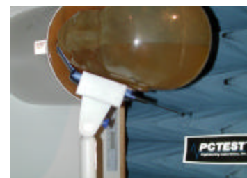
Figure 15. Head SAR Test Setup
