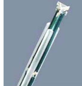
Figure 3.4 Probe Thick-Film Technique
