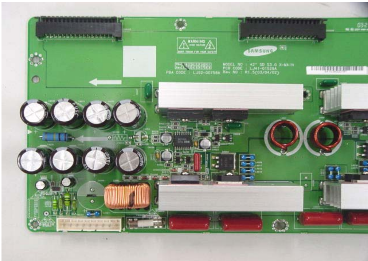
X driver board top view
