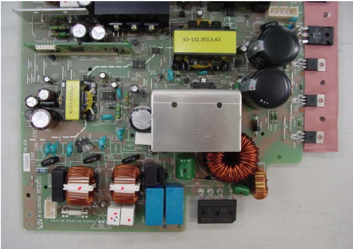
SMPS board-2 top view
