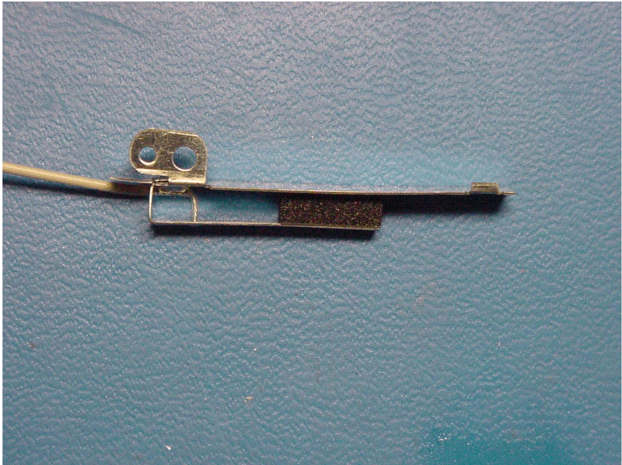
PHOTOGRAPH 7: MAIN ANTENNA (GEMINI 2)
