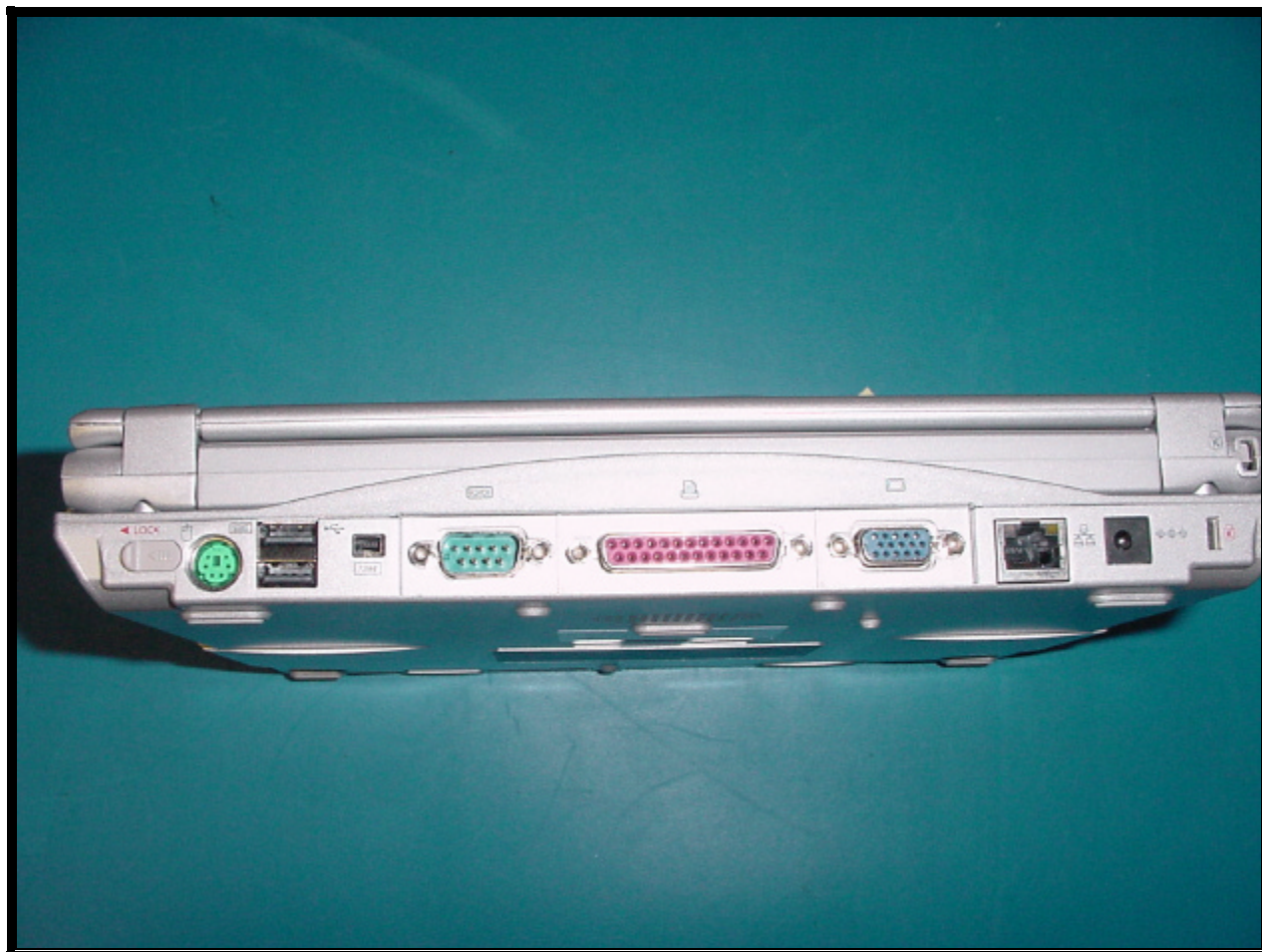
PHOTOGRAPH 7: REAR OF HOST WITH I/O PORTS
