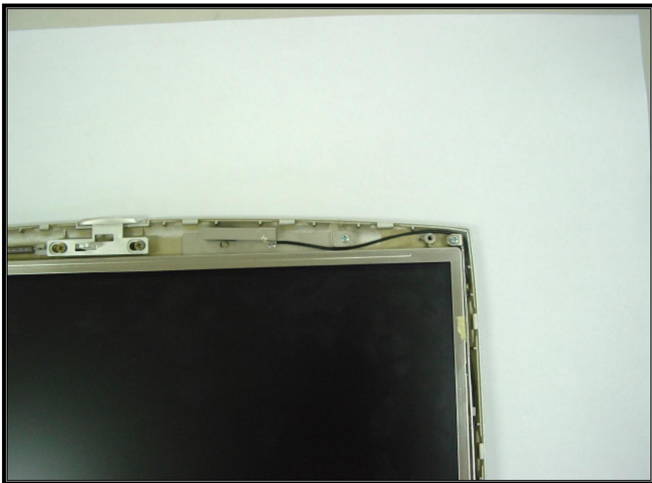
PHOTOGRAPH 10: TOP VIEW OF MAIN TRANSMITTING ANTENNA
