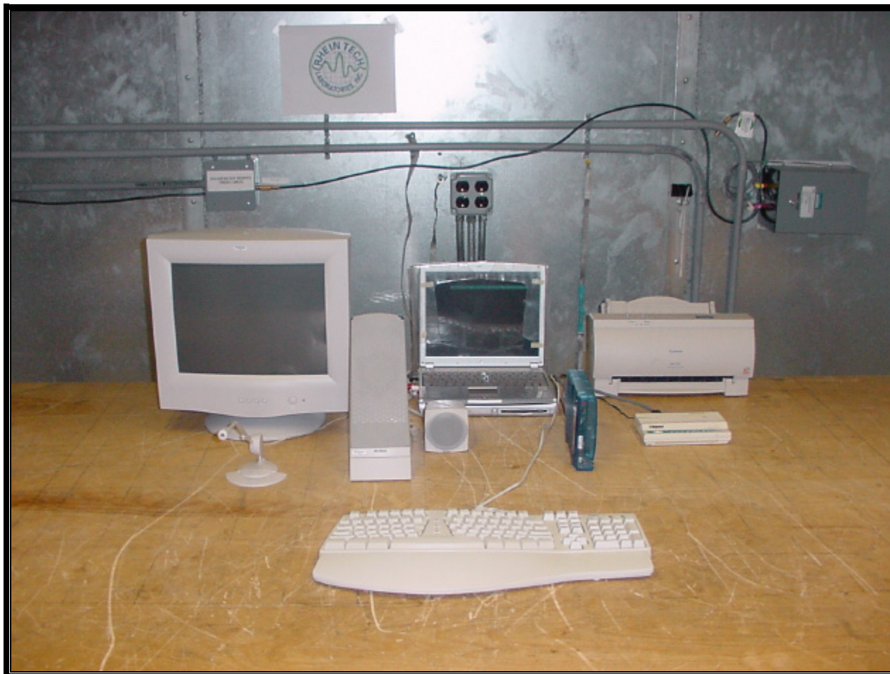
PHOTOGRAPH 1: CONDUCTED EMISSION FRONT VIEW WORST CASE CONFIGURATION
