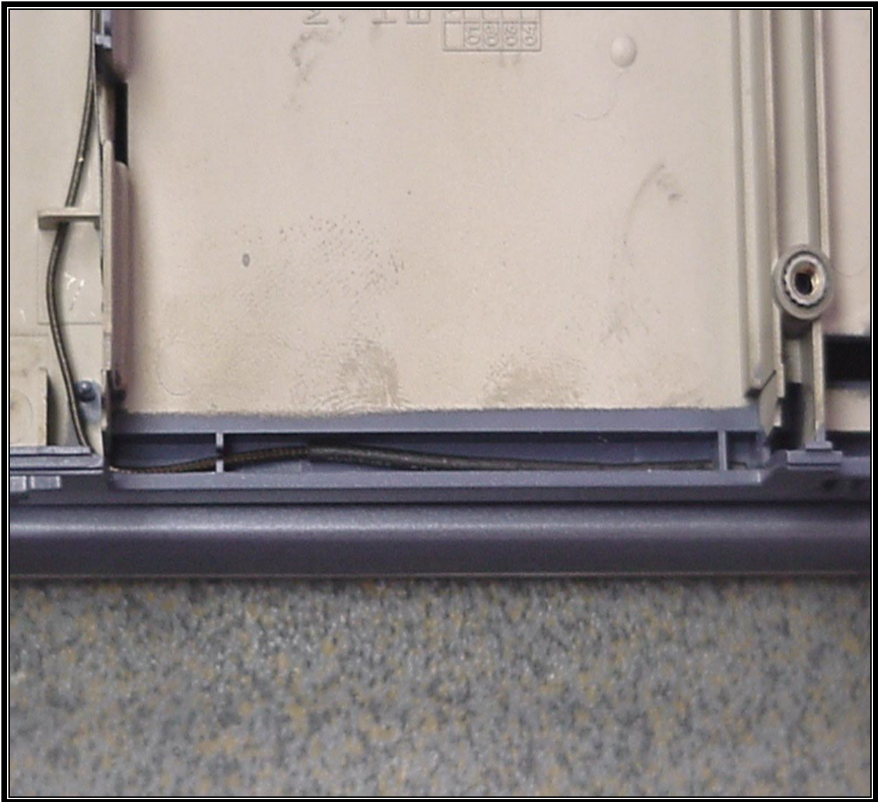
PHOTOGRAPH 8: MAIN TX/RX ANTENNA (DIPOLE)
