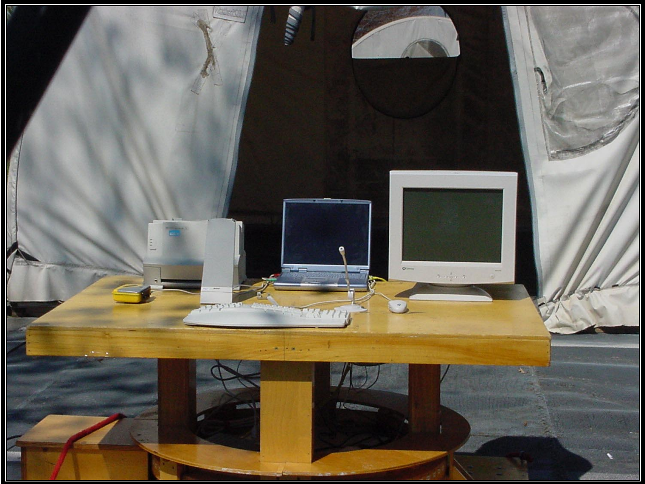
PHOTOGRAPH 2: RADIATED EMISSION FRONT VIEW WORST CASE CONFIGURATION
