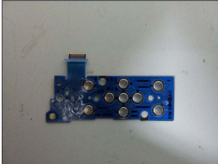
Top view of keypad PCB
