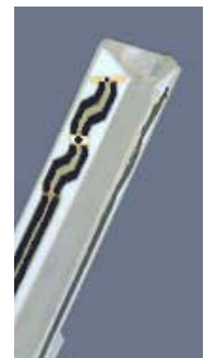
Figure 4.2 Probe Thick-Film Technique
