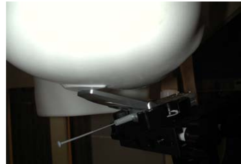
Figure 15.5 Right Head SAR Test Setup -- Ear / 15° Tilt Position --
