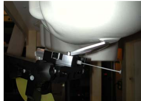
Figure 15.5 Left Head SAR Test Setup -- Ear / 15° Tilt Position --
