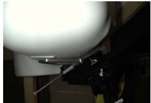
Figure 15.5 Right Head SAR Test Setup -- Cheek / Touch Position --
