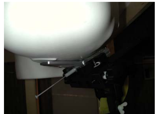
Figure 15.1 Right Head SAR Test Setup -- Cheek / Touch Position --
