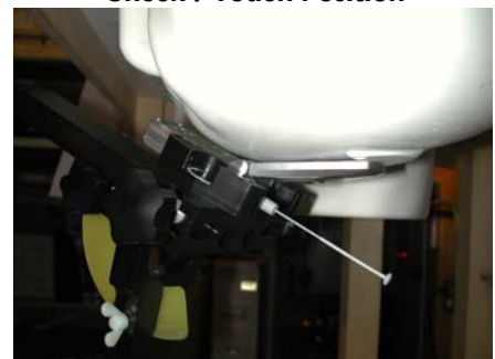
Figure 15.3 Left Head SAR Test Setup -- Cheek / Touch Position --
