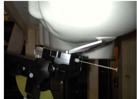
Figure 15.4 Left Head SAR Test Setup -- Ear / 15° Tilt Position --
