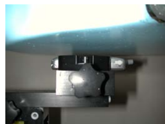
Figure 27. Body SAR Test Setup
