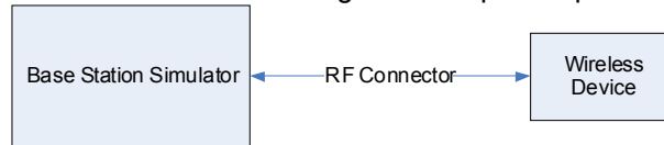
Figure 8-2 Power Measurement Setup
