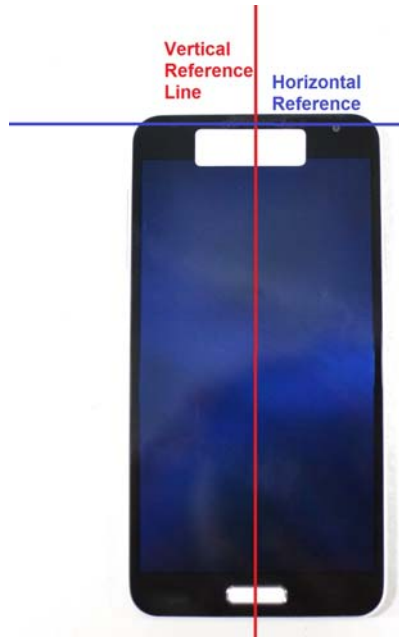
SAR Test Setup Photo 11: Horizontal and Vertical Reference Lines
