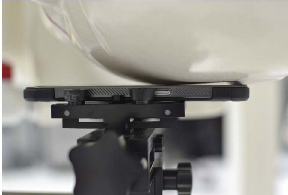
SAR Test Setup Photo 3: Left Cheek
