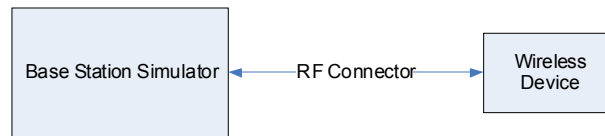
Figure 11-1 Power Measurement Setup
