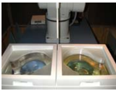
Figure 5.2 Head Simulated Tissue
