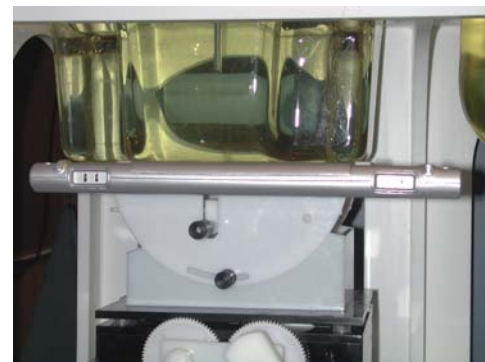
Figure 14.1 DSSS Body SAR Test Setup
