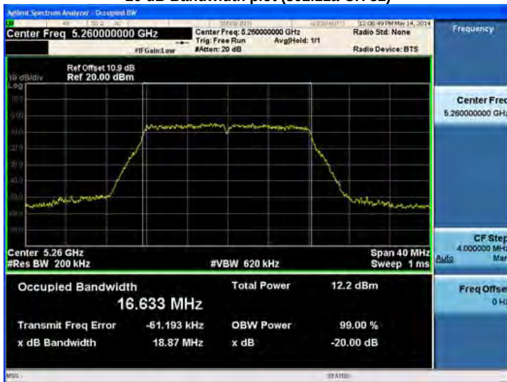
20 dB Bandwidth plot (802.11a-CH 52)
