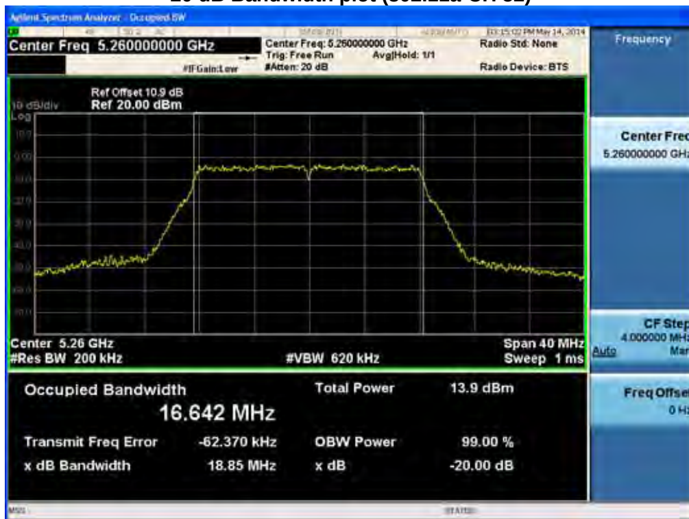
20 dB Bandwidth plot (802.11a-CH 52)
