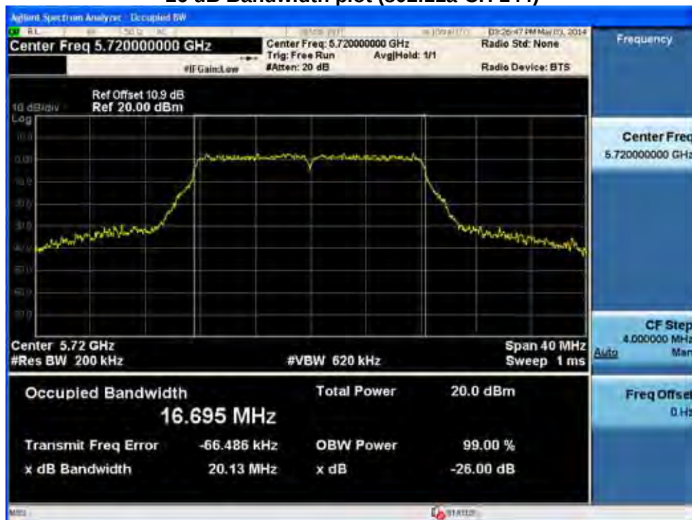
26 dB Bandwidth plot (802.11a-CH 144)
