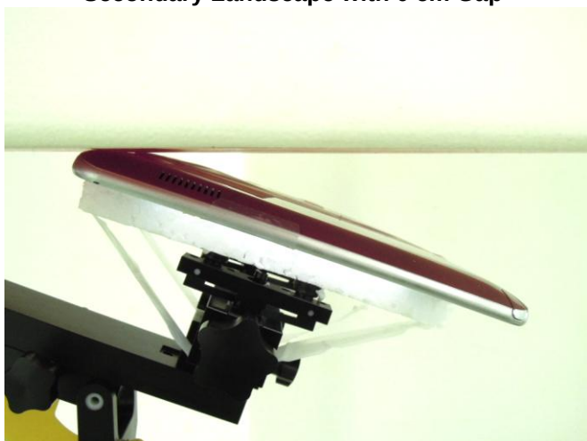
Rear Face of EUT with 0 cm Gap (Top Edge/Left Rear Corner at 20 degree)
