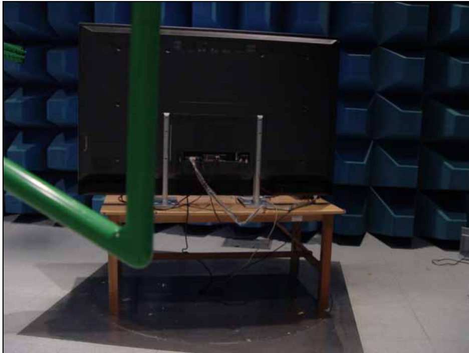
Picture 3. Radiated Emission (rear view)
