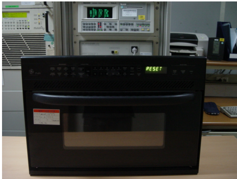
Fig.3 Test Setup for RF output power
