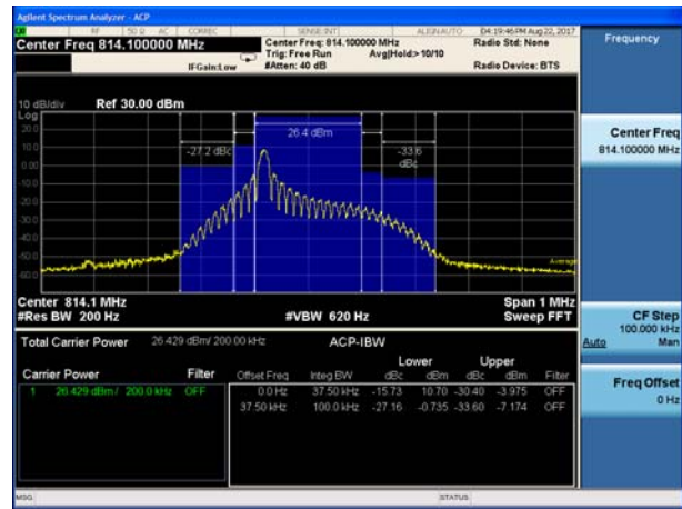
NB-IOT Band 26 BPSK 15kHz 1@6 CH-Middle
