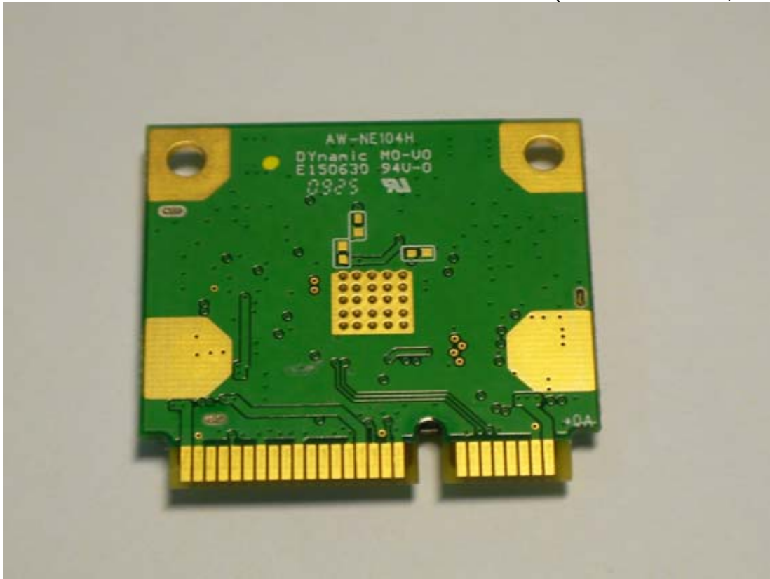
Figure 15 Internal View (Wireless Module, Back View)
