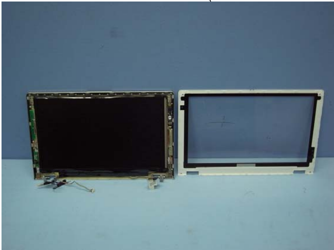
Figure 28 Internal View (Front Cover & LCD Panel Removed)
