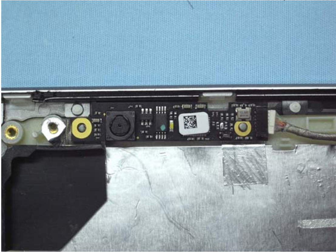
Figure 29 Internal View (Web Camera View)
