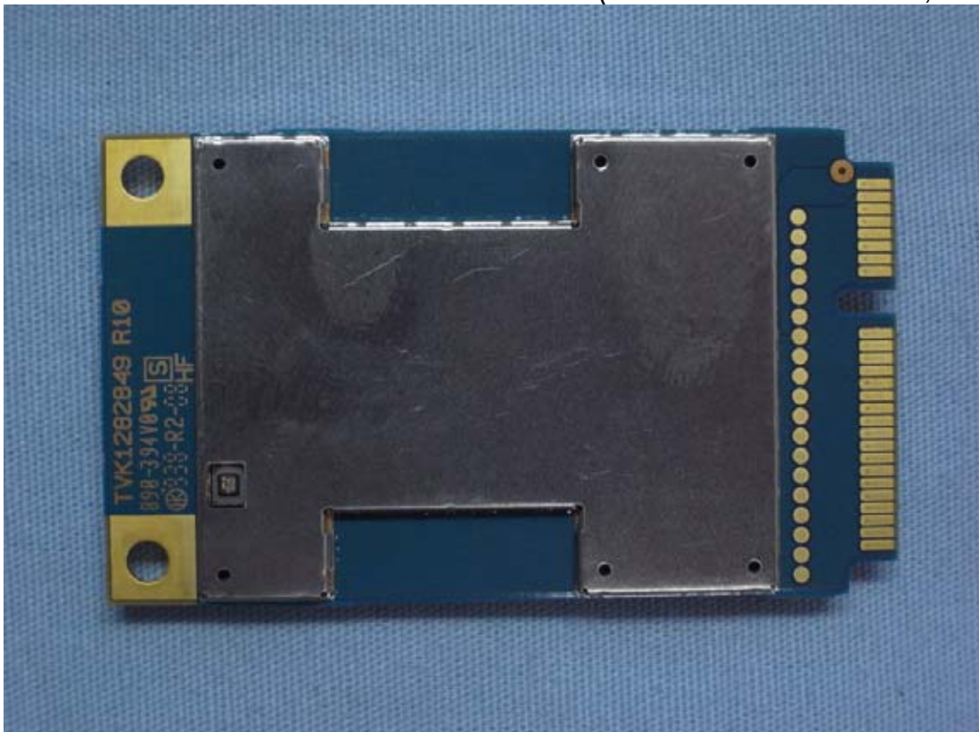
Figure 26 Internal View (Mobil Broadband Module, Back View)
