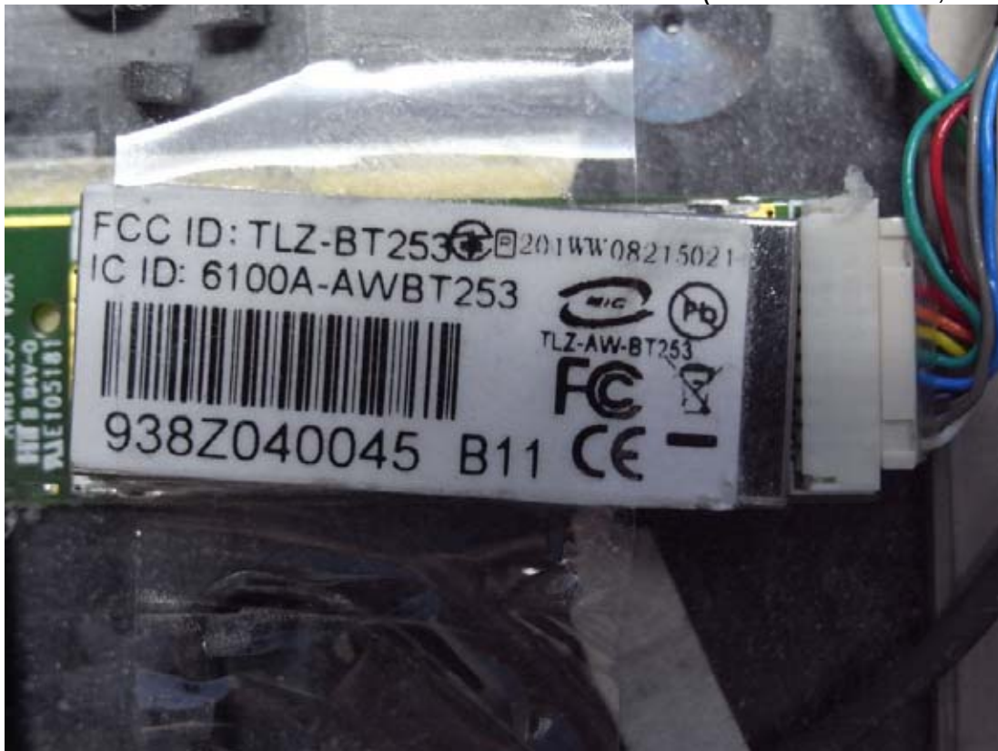
Figure 19 Internal View (Bluetooth Module, Label View)
