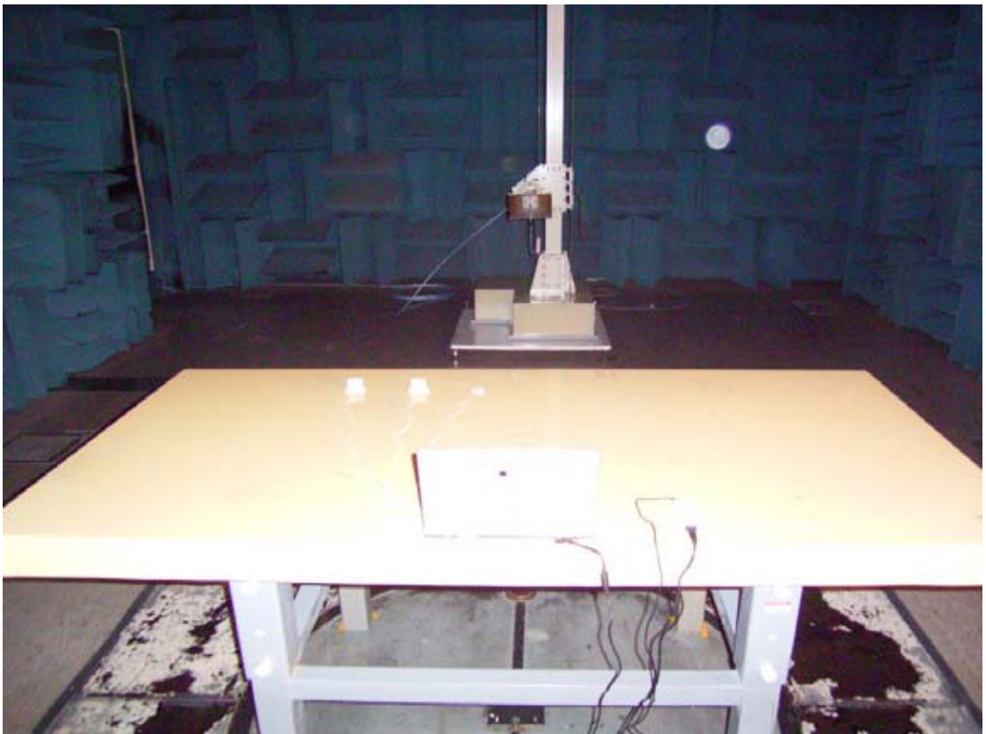
BACK VIEW OF RADIATED MEASUREMENT
