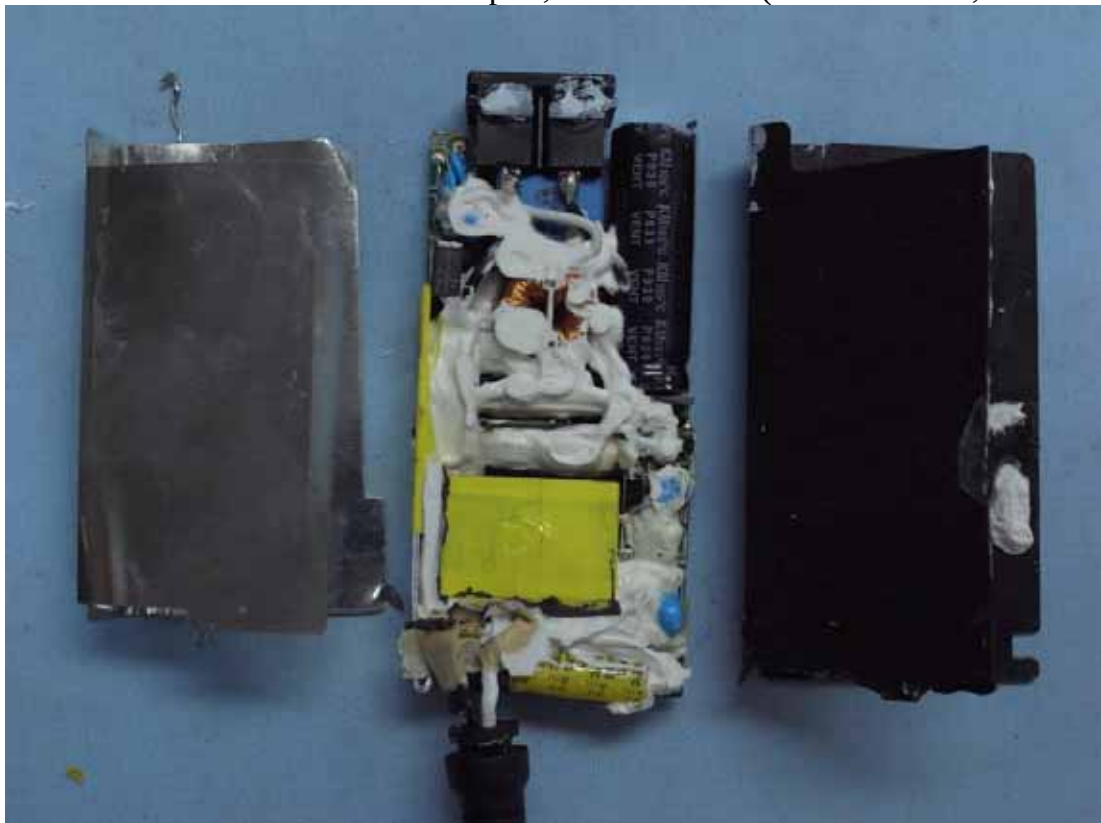
Figure 49 AC Adapter, Internal View (Control Board, Front View)
