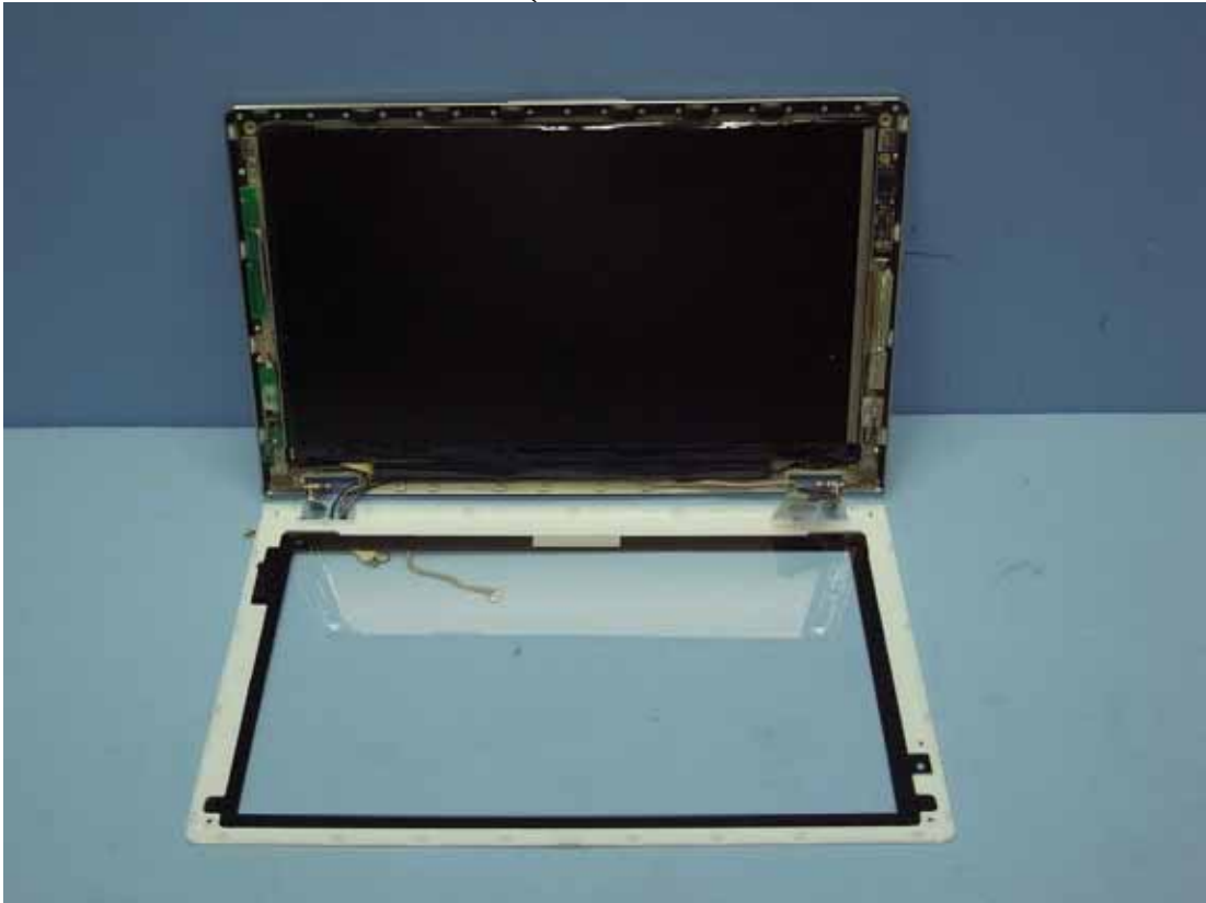
Figure 35 Internal View (Removed Front Frame, LCD Panel/Front View)
