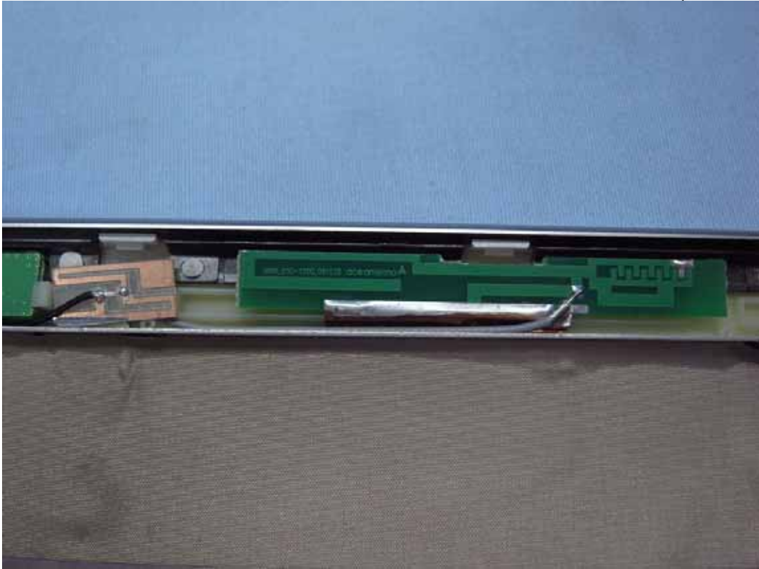
Figure 42 Mobil Broadband & Wireless LAN Antenna (Back View)
