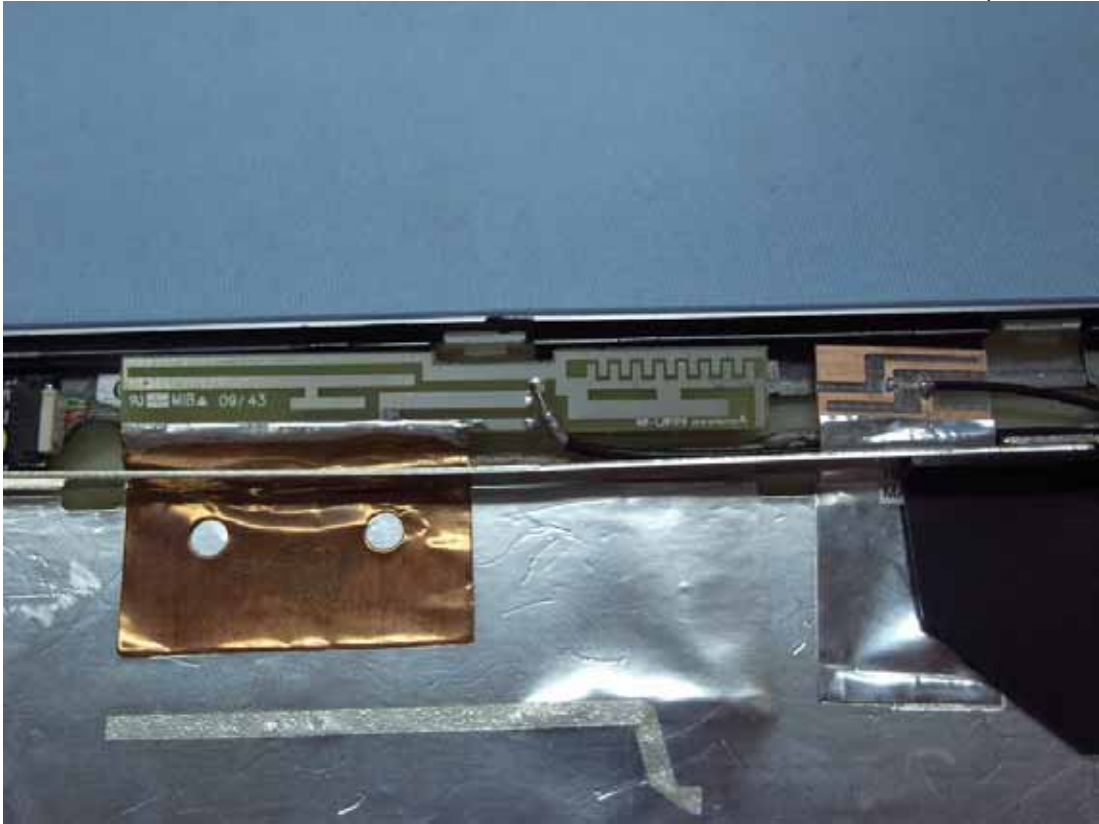
Figure 38 Mobil Broadband & Wireless LAN Antenna (Back View)
