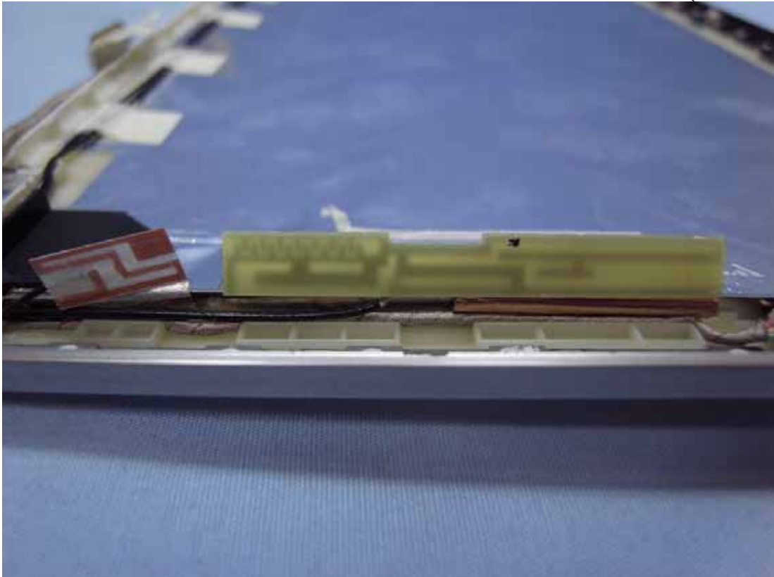
Figure 39 Mobil Broadband & Wireless LAN Antenna (Front View)
