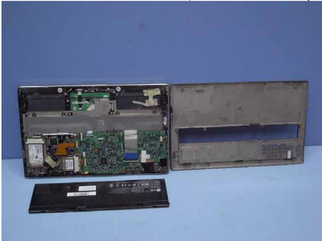
Figure 10 Internal View (Removed Case Covers & Keyboard)
