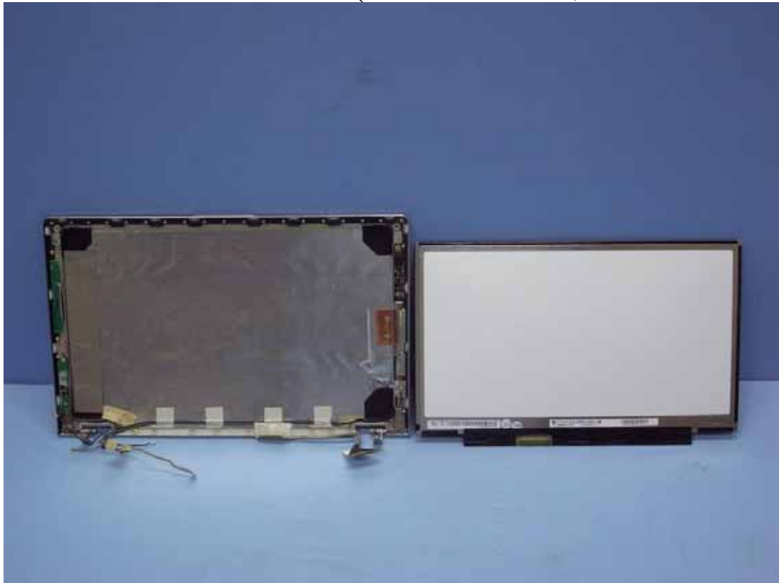
Figure 36 Internal View (Removed LCD Panel, LCD Panel/Back View)
