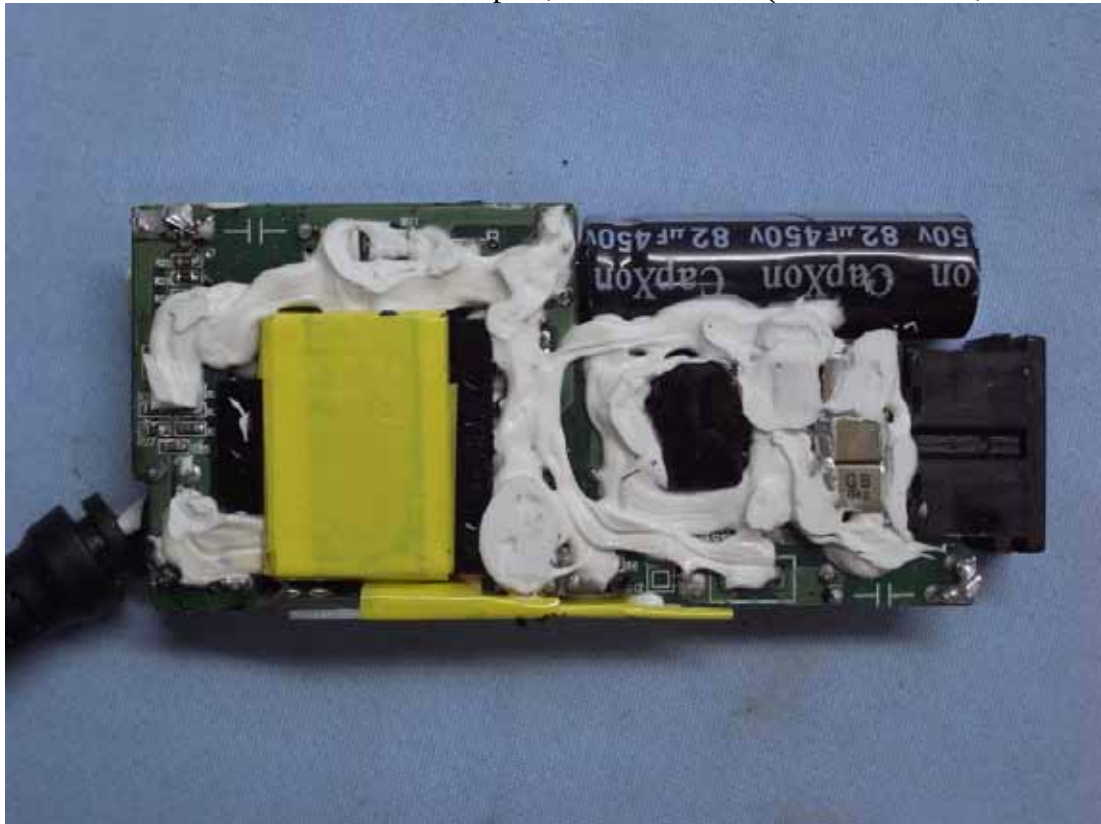
Figure 50 AC Adapter, Internal View (Control Board, Back View)
