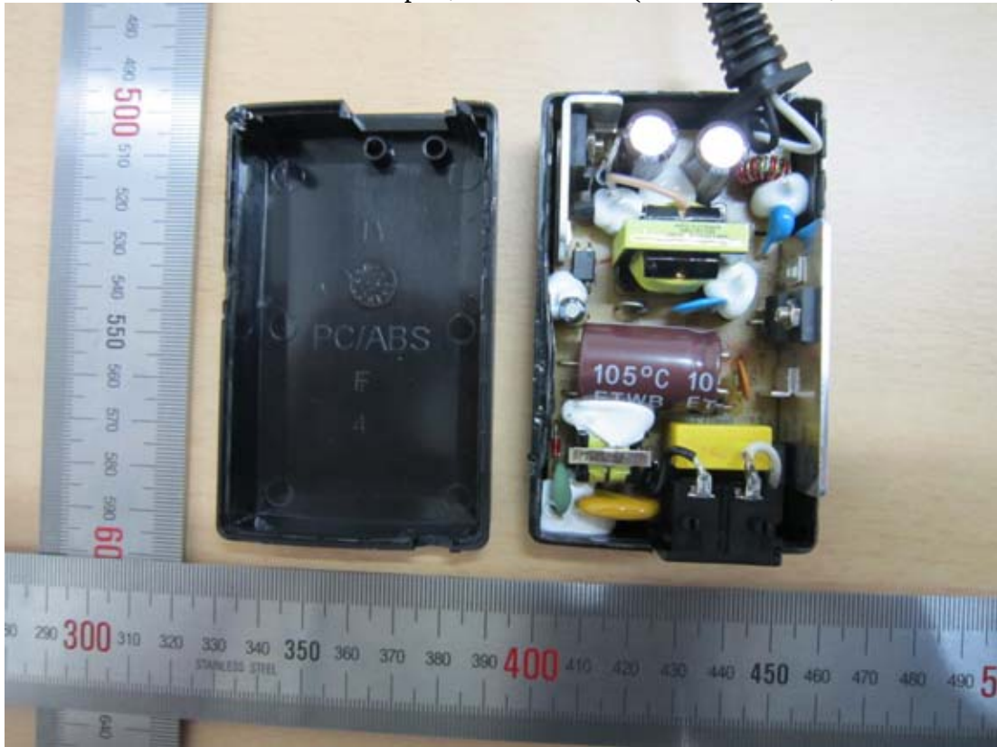
Figure 11 AC Adapter, Internal View (Removed Cover, PCB/Front View)
