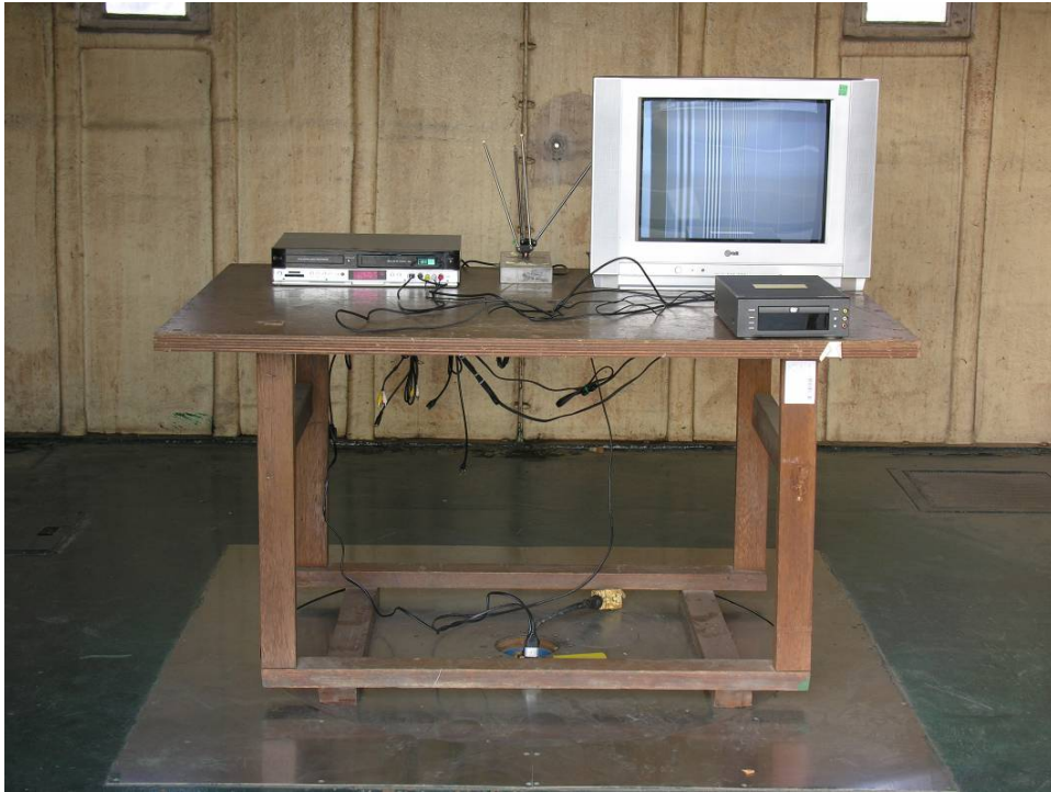
Photographs of Test Set-up (Radiated emissions)
