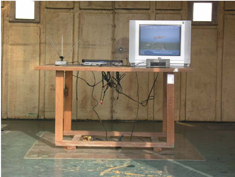
Photographs of Test Set-up (Radiated emissions)
