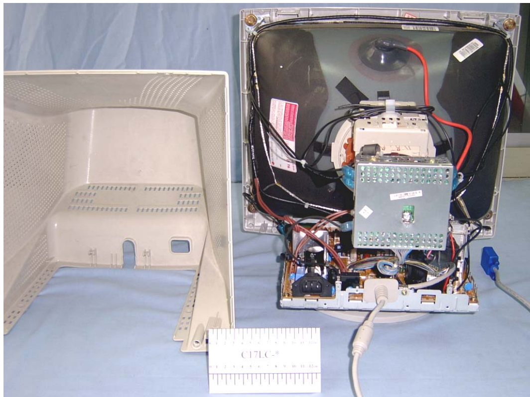
FIGURE 1 COLOR MONITOR (M/N:C17LC-*) COVER REMOVED 1
