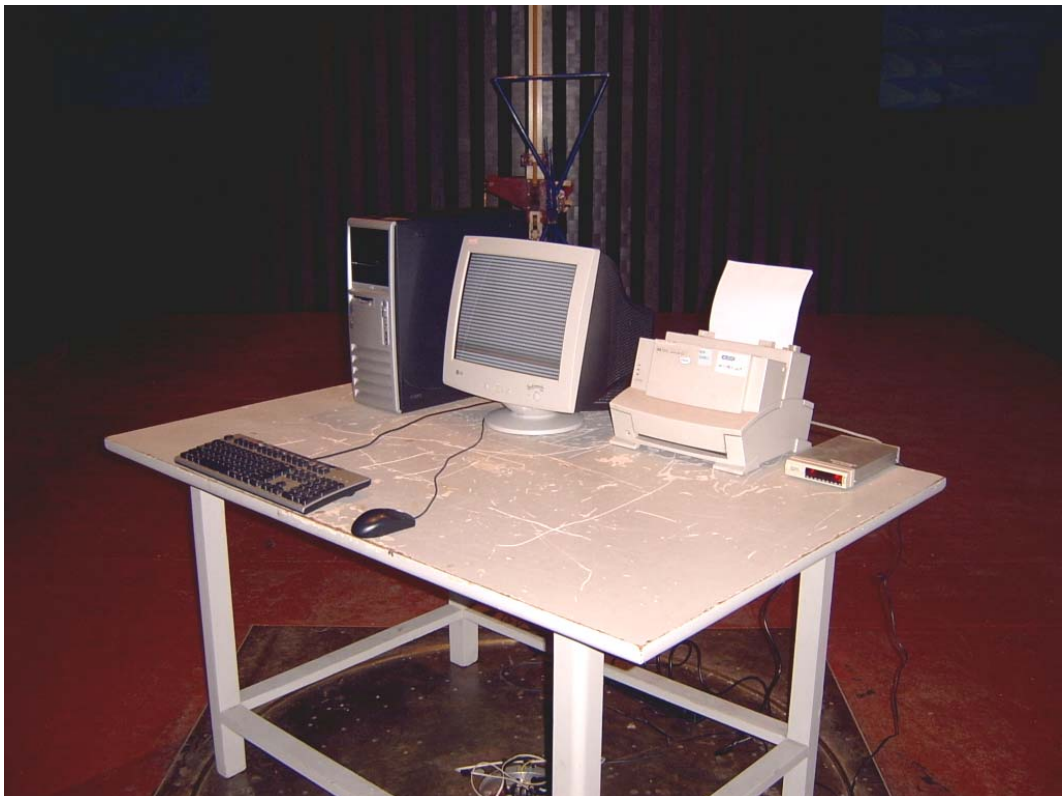
SETUP WITH MAXIMUM DETECTED EMISSION AT VERTICAL POLARIZATION (1280*1024 60Hz MODE)
