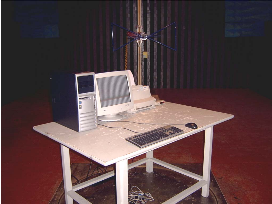
SETUP WITH MAXIMUM DETECTED EMISSION AT HORIZONTAL POLARIZATION (1280*1024 60Hz MODE)
