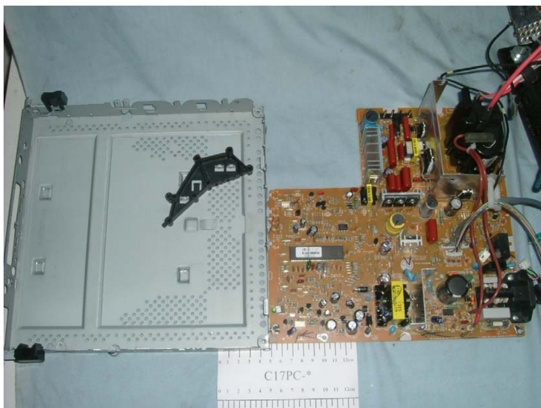
FIGURE 10 CRT MONITOR (M/N: C17PC-*) MAIN BOARD 1 COVER REMOVED
