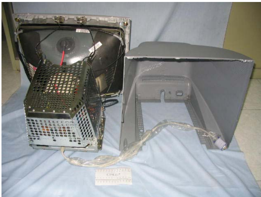
FIGURE 1 COLOR MONITOR (M/N:C19LE-*) COVER REMOVED #1
