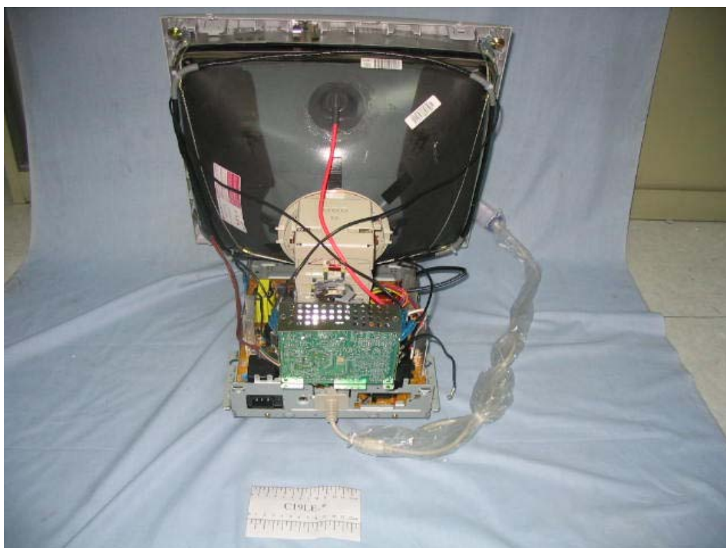
FIGURE 2 COLOR MONITOR (M/N:C19LE-*) COVER REMOVED #2
