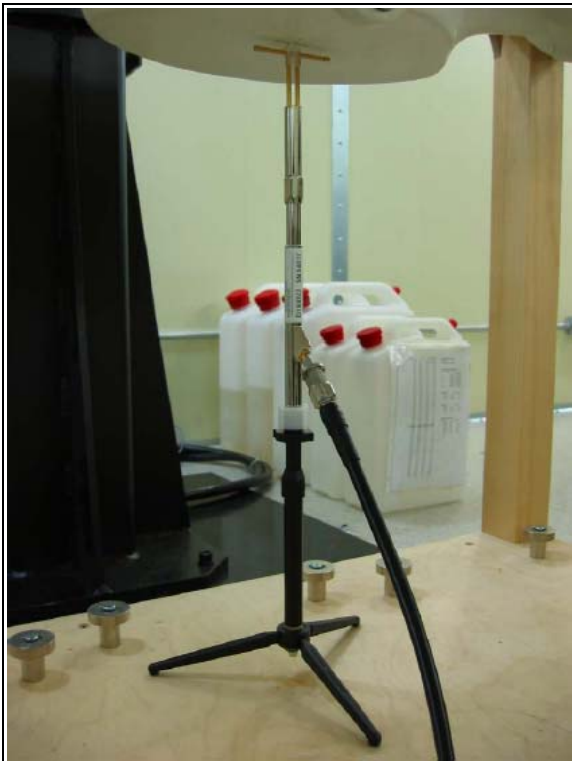
Figure 2 1900 MHz Dipole Validation Test Setup
