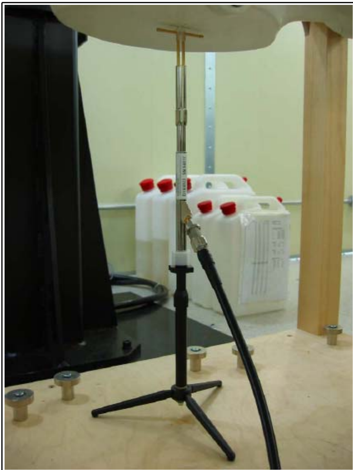
Figure 2 1900 MHz Dipole Validation Test Setup
