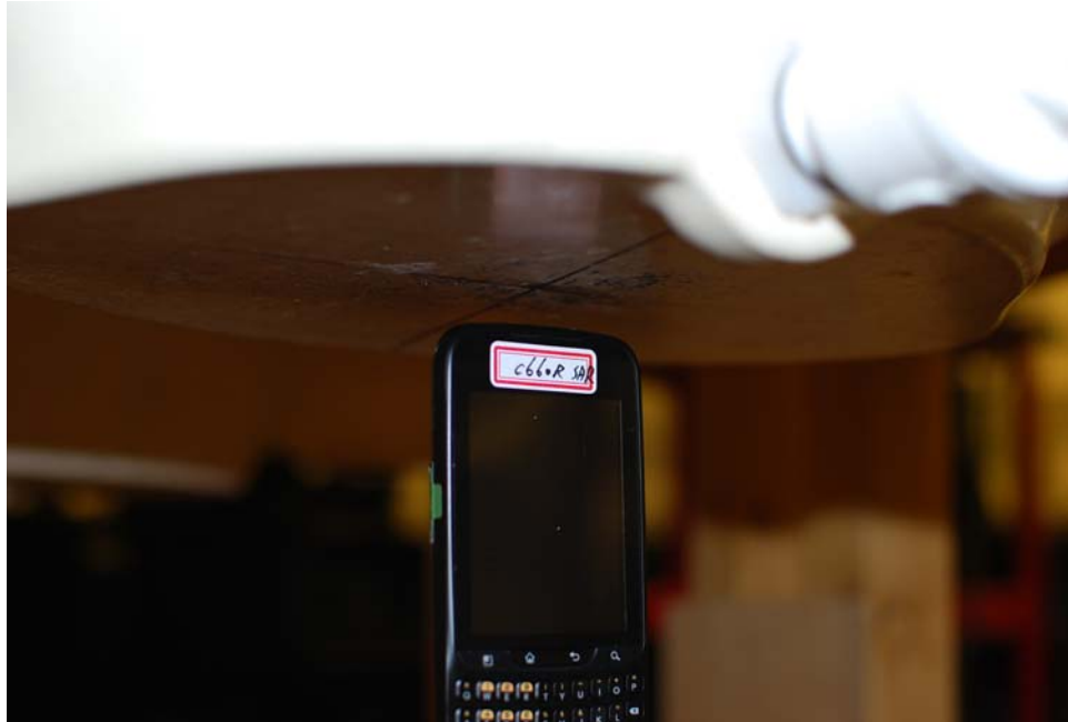
SAR Test Setup Photo 7: Top at 1.0 cm
