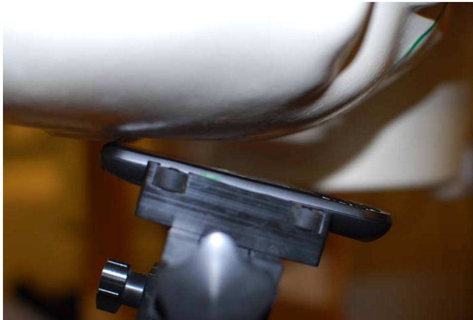
SAR Test Setup Photo 2: Right Tilt
