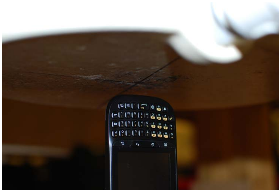
SAR Test Setup Photo 8: Bottom at 1.0 cm
