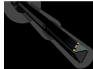
Figure 4-3 Triangular Probe Configuration
