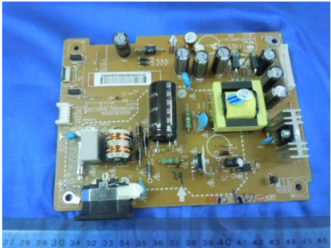
FIGURE 6 LCD MONITOR (M/N: D2242PY) POWER BOARD (COMPONENT SIDE)
