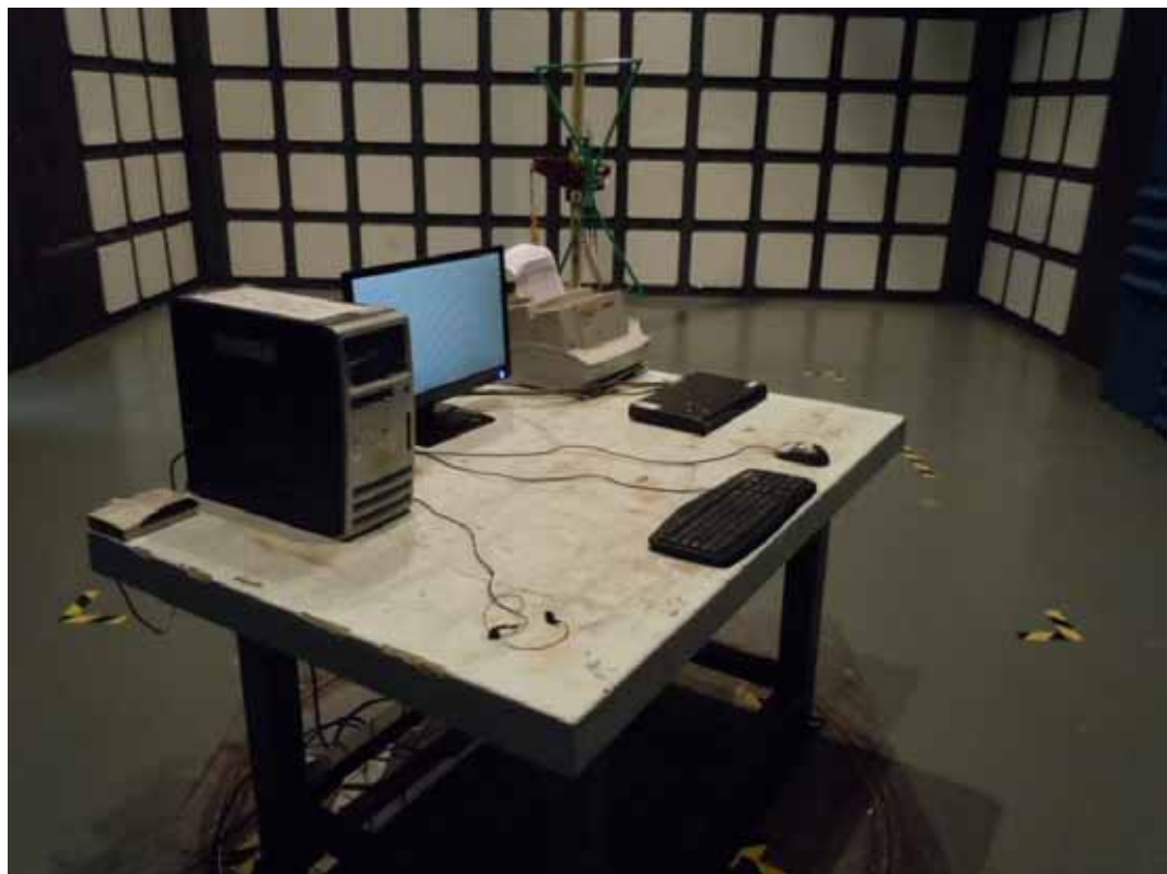
SETUP WITH MAXIMUM DETECTED EMISSION AT VERTICAL POLARIZATION (TEST MODE: DVI 640*480@60Hz)
