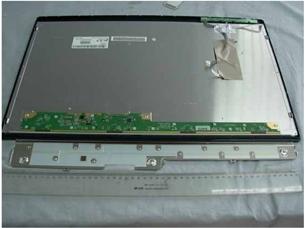
FIGURE 8 LCD MONITOR (M/N: D2341PY) DISPLAY BOARD (COMPONENT SIDE)
