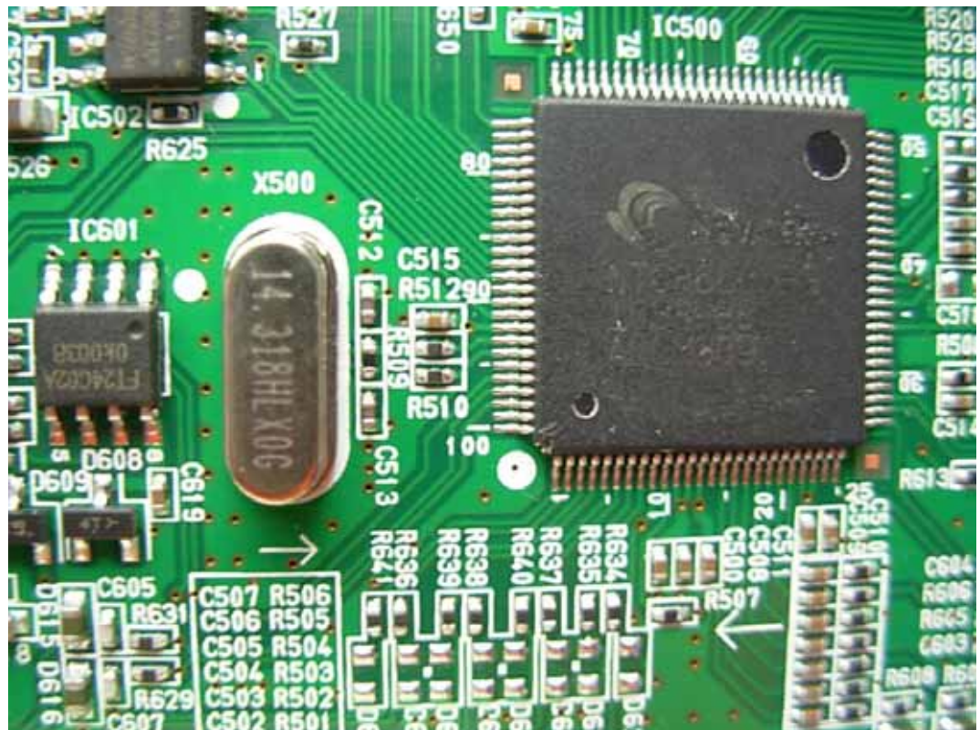
FIGURE 7 LCD MONITOR (M/N: D2341PY) CHIP & CRYSTAL ON MAIN BOARD
