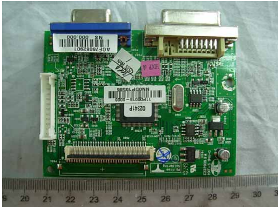
FIGURE 5 LCD MONITOR (M/N: D2341PY) MAIN BOARD (COMPONENT SIDE)
