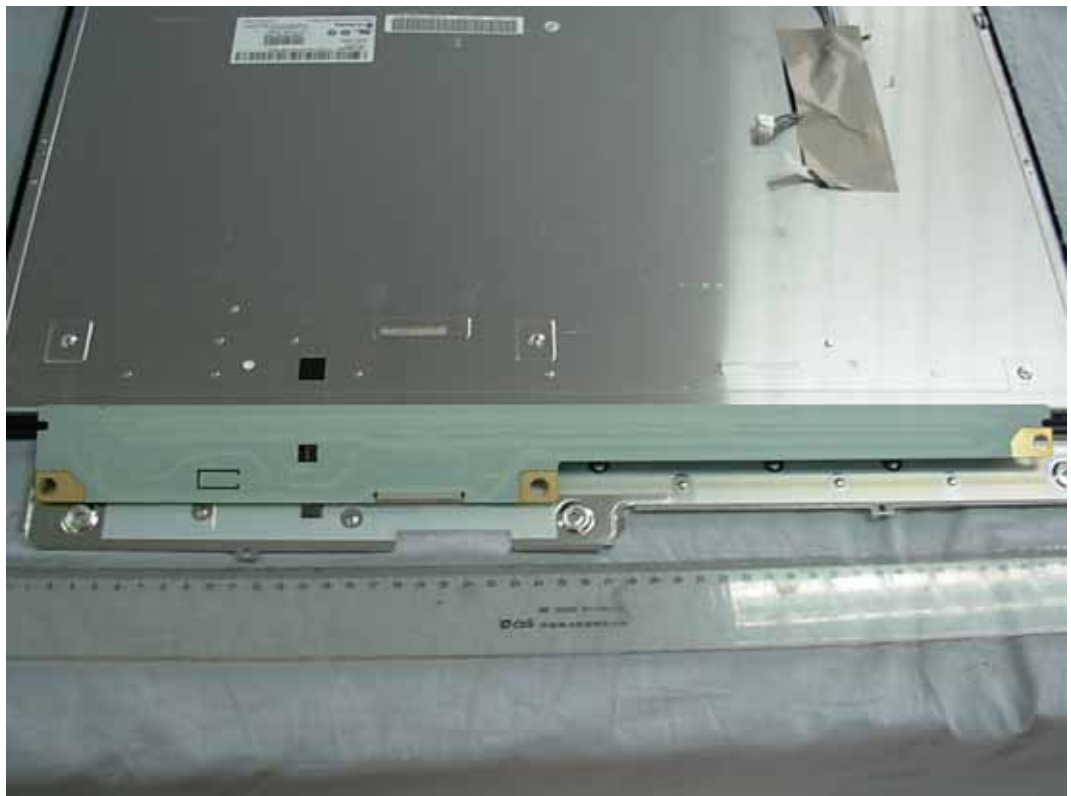
FIGURE 9 LCD MONITOR (M/N: D2341PY) DISPLAY BOARD (SOLDERED SIDE)
