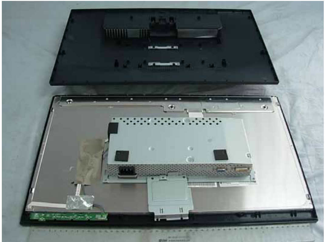
FIGURE 1 LCD MONITOR (M/N: D2341PY) COVER REMOVED
