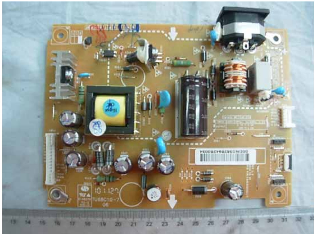
FIGURE 3 LCD MONITOR (M/N: D2341PY) POWER BOARD (COMPONENT SIDE)
