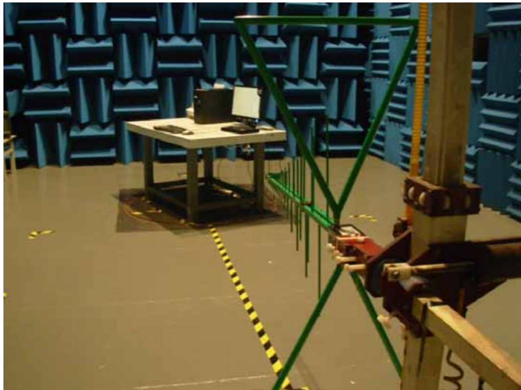
SETUP WITH MAXIMUM DETECTED EMISSION AT VERTICAL POLARIZATION (TEST MODE: DVI 1280*1024@60Hz)
