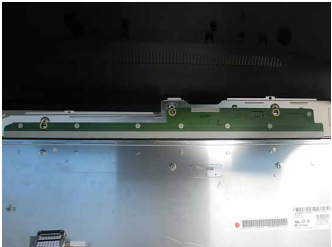
FIGURE 9 LCD MONITOR (M/N: D2542PY) DISPLAY BOARD (SOLDERED SIDE)
