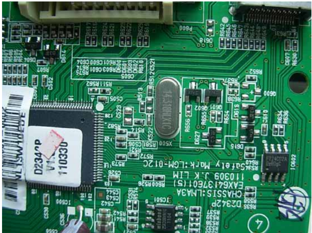
FIGURE 5 LCD MONITOR (M/N: D2542PY) CHIP & CRYSTAL ON MAIN BOARD
