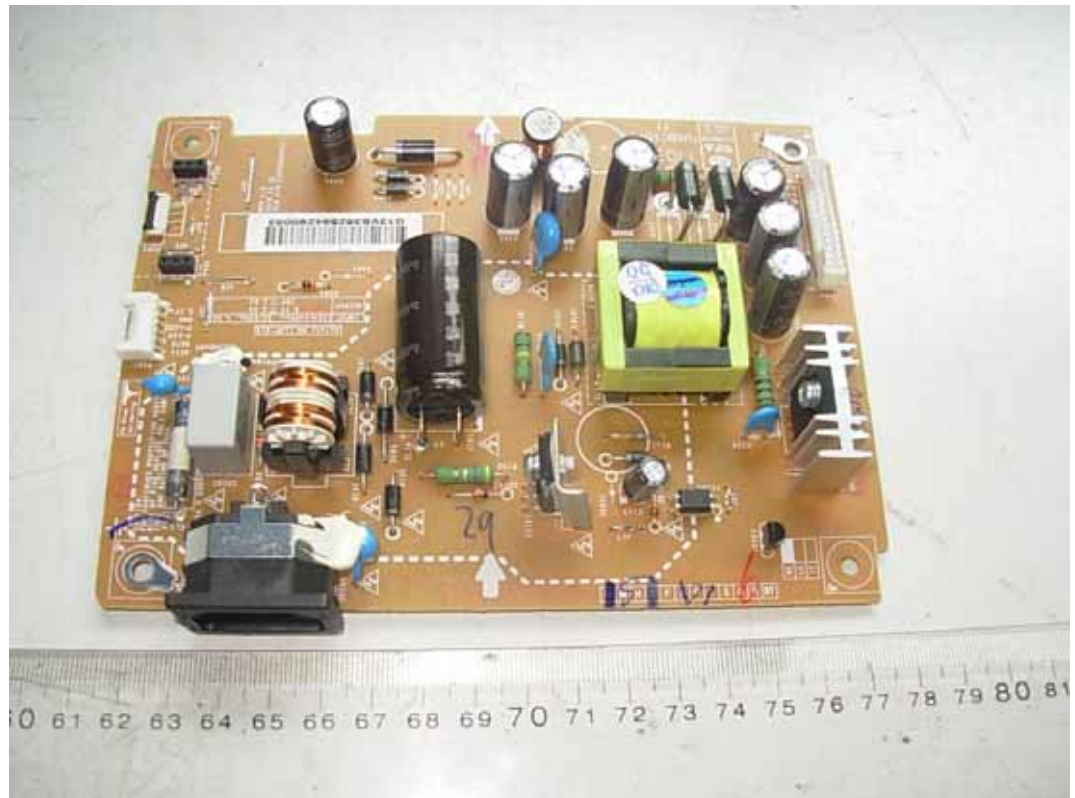
FIGURE 6 LCD MONITOR (M/N: D2542PY) POWER BOARD (COMPONENT SIDE)
