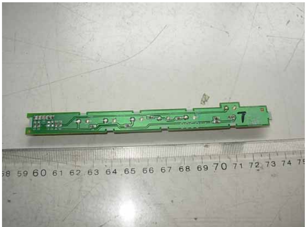
FIGURE 11 LCD MONITOR (M/N: D2542PY) KEY BOARD (SOLDERED SIDE)
