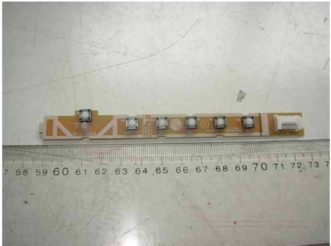
FIGURE 10 LCD MONITOR (M/N: D2542PY) KEY BOARD (COMPONENT SIDE)
