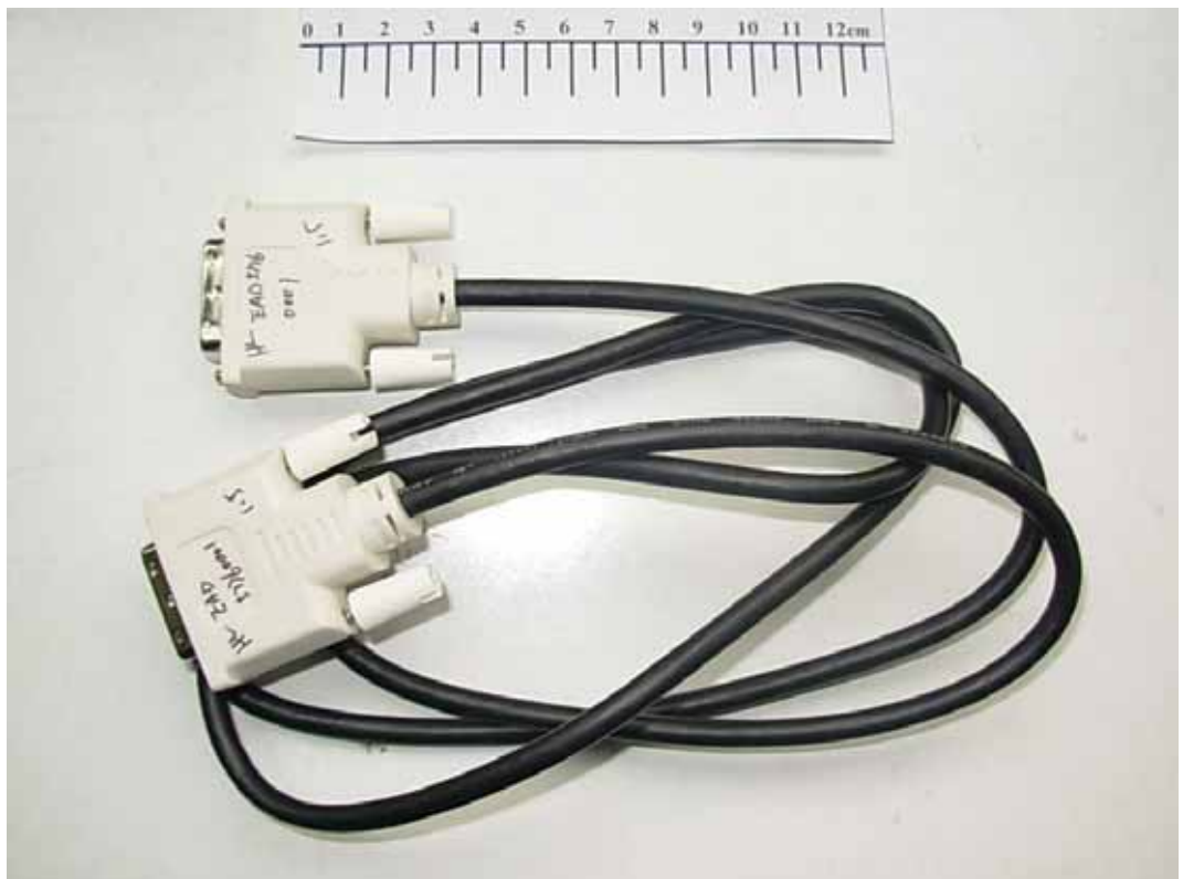
FIGURE 10 LCD MONITOR (M/N: E1910PMW) DVI CABLE #2
