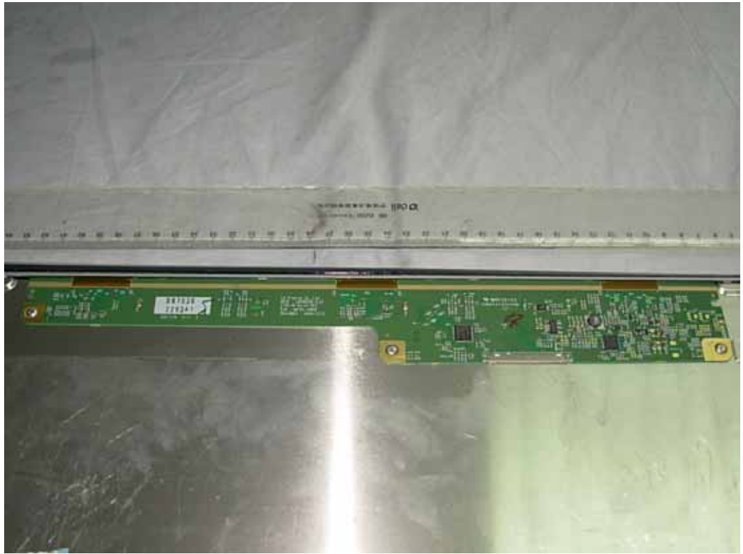
FIGURE 8 LCD MONITOR (M/N: E1910PMW) DISPLAY BOARD (COMPONENT SIDE)
