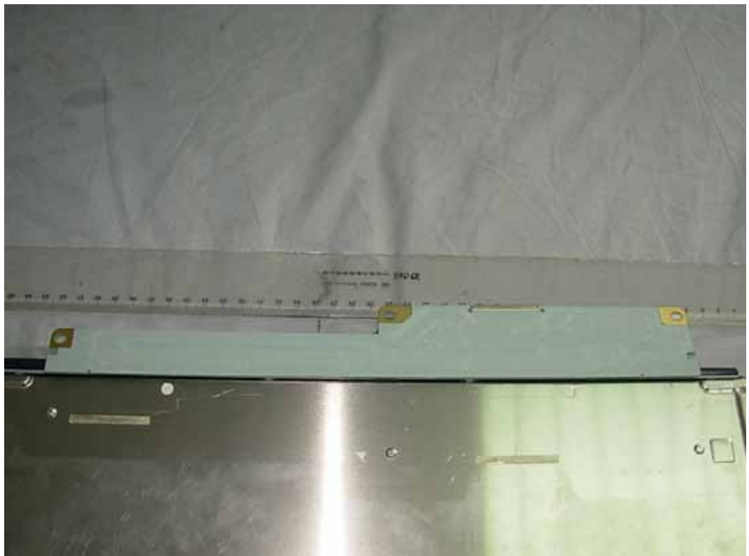
FIGURE 9 LCD MONITOR (M/N: E1910PMW) DISPLAY BOARD (SOLDERED SIDE)
