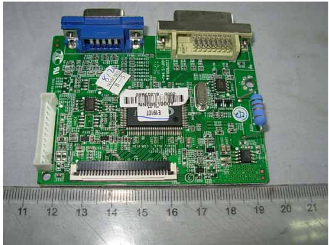
FIGURE 5 LCD MONITOR (M/N: E1910PW) MAIN BOARD (COMPONENT SIDE)
