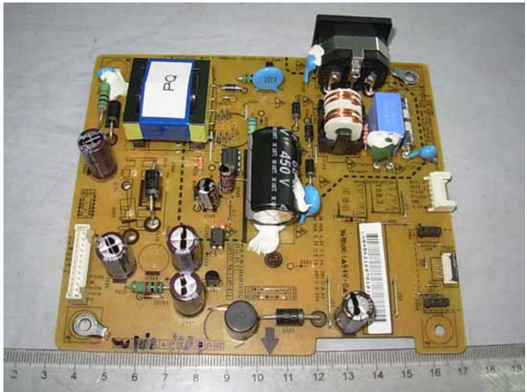
FIGURE 3 LCD MONITOR (M/N: E1910PW) POWER BOARD (COMPONENT SIDE)
