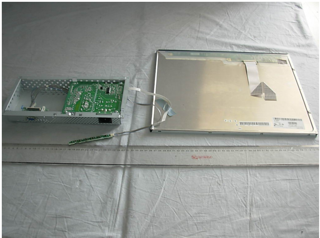
FIGURE 2 LCD MONITOR (M/N: E1910SW) POWER BOX REMOVED
