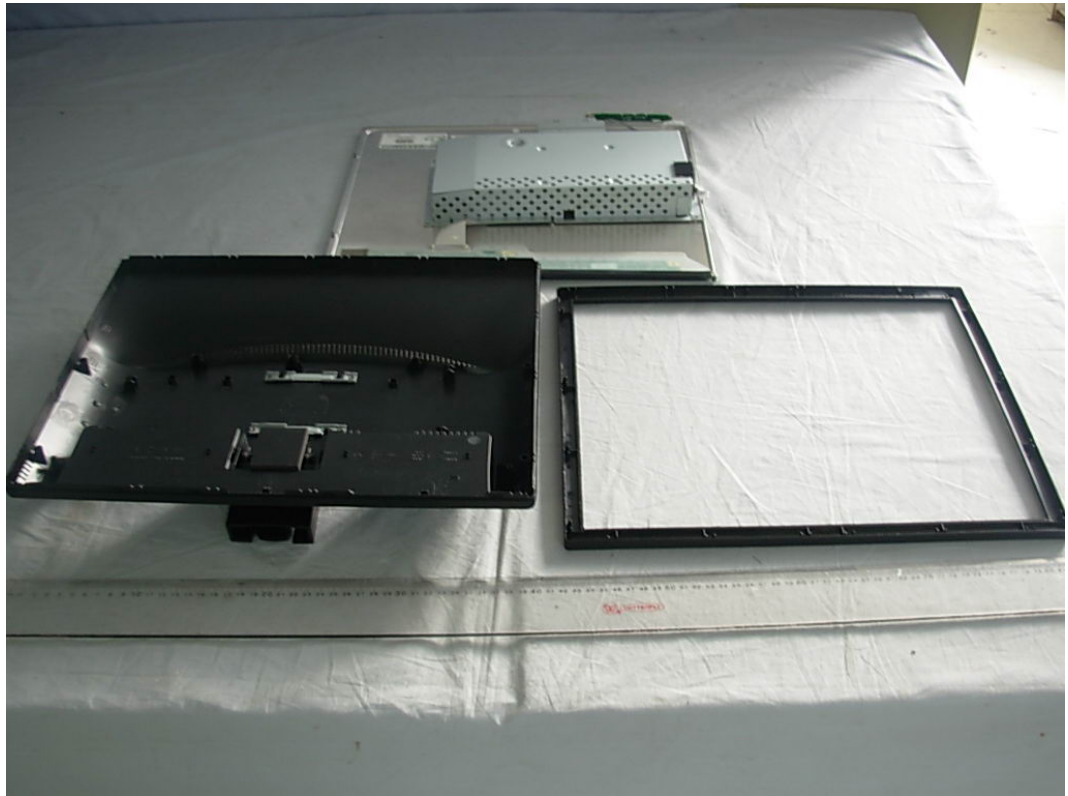
FIGURE 1 LCD MONITOR (M/N: E1910SW) COVER REMOVED
