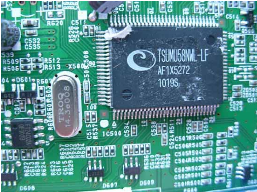
CHIP & CRYSTAL ON MAIN BOARD
