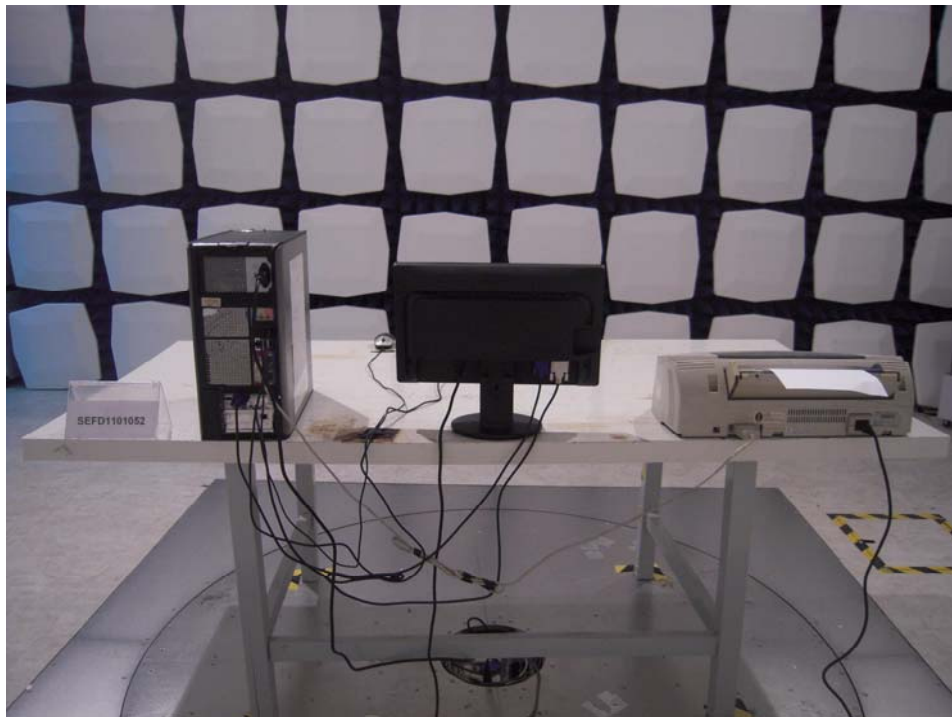
Back View of Radiated Emission Test
