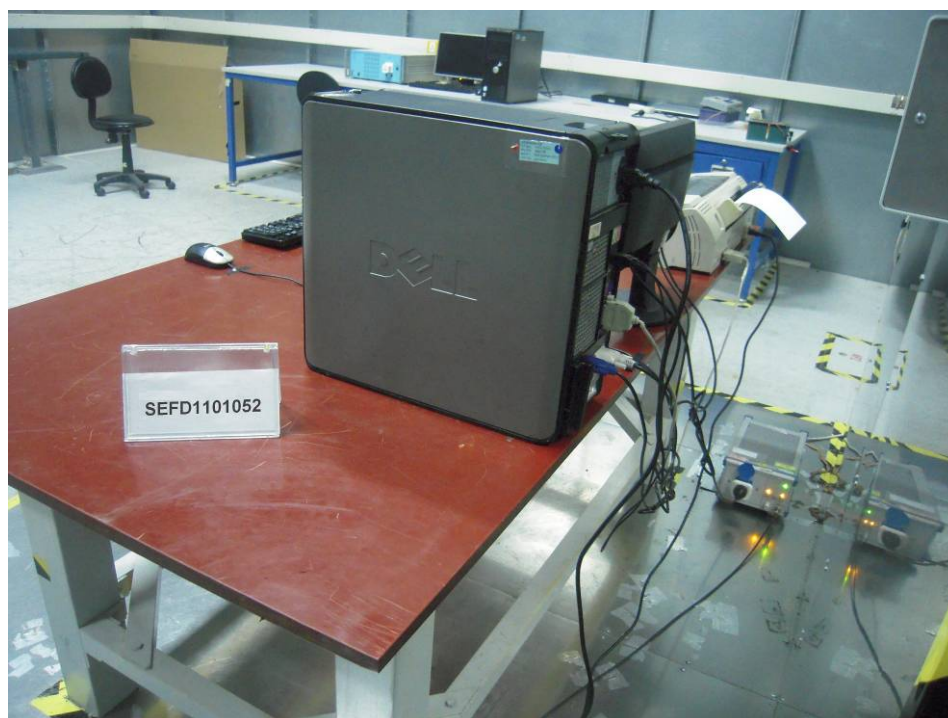
Back View of Conducted Emission Test
