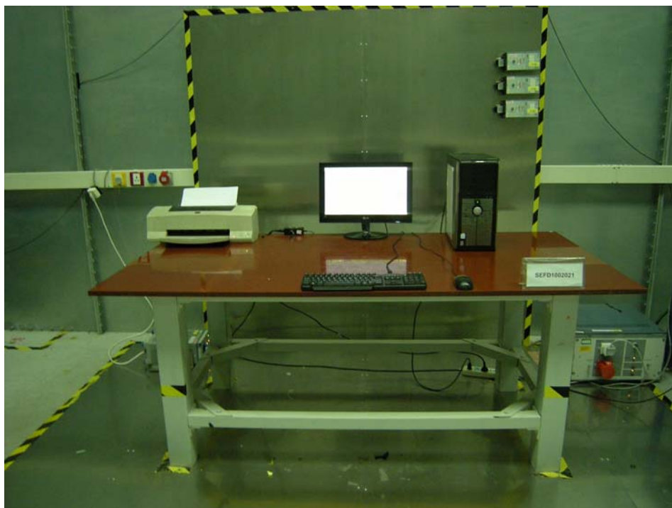
Front View of Conducted Emission Test
