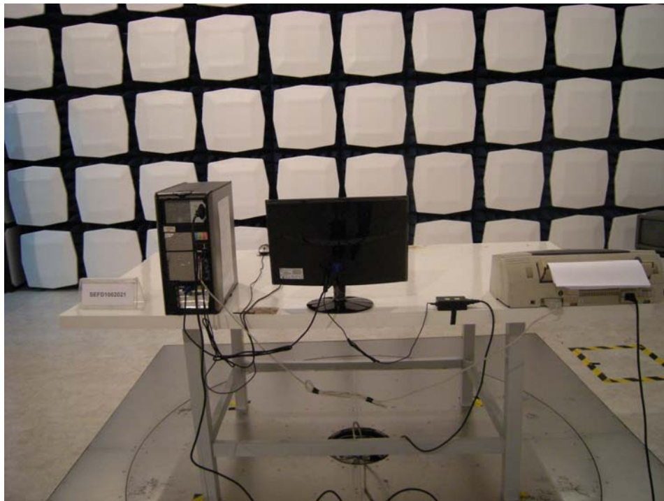
Back View of Radiated Emission Test
