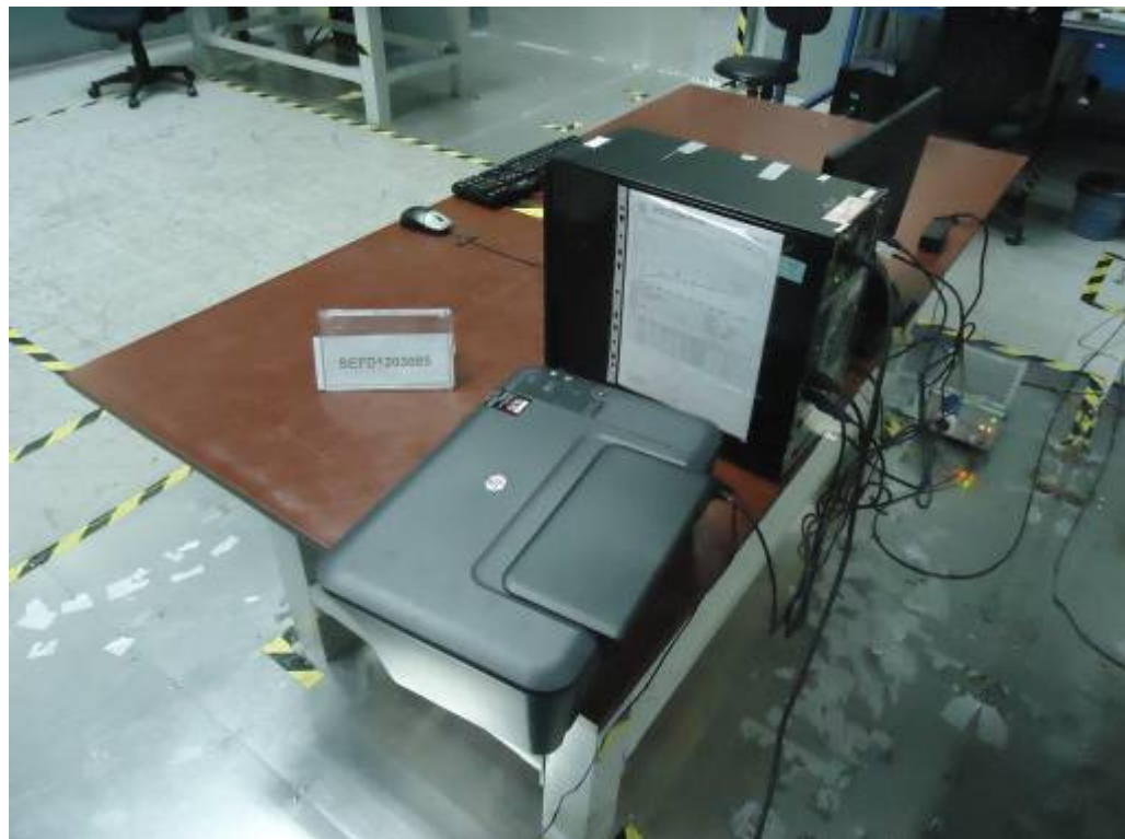
Back View of Conducted Emission Test
